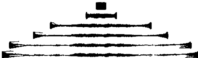
FIG. 13. Sequence of filament shapes in a constant-strain-rate deformation at \dot{\epsilon}_0 = 0.004\tau^{-1} , at times 0, 295\tau, 595\tau, 668\tau, 743\tau, and 763\tau .
